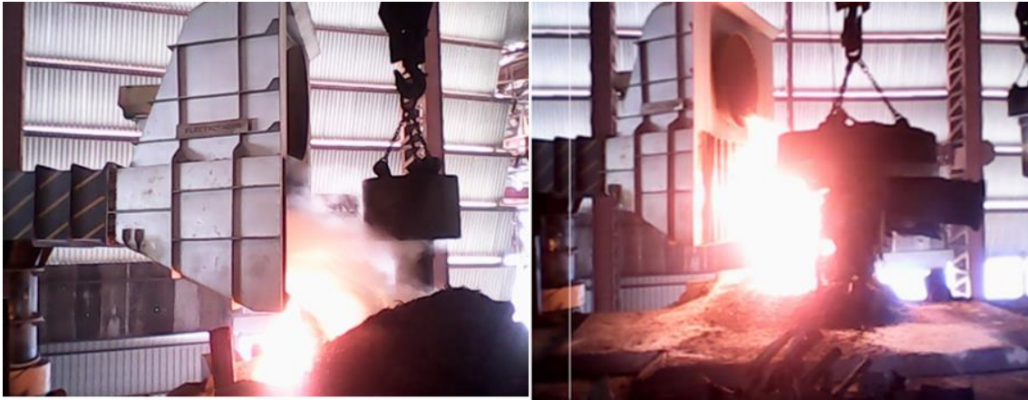
Figure 6.13: Working of side-based Suction Hood
