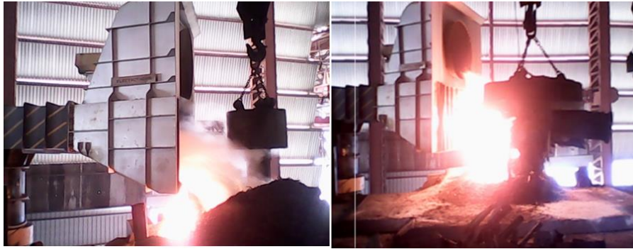
Figure 6.11: Working on side-based Suction Hood (Sharma, 2020)
