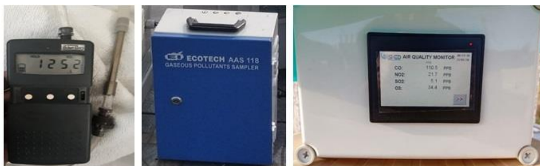
(g) Low flow pump (h) gaseous sampler (i) Online gas analyzer
